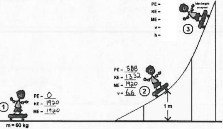
Calculate the potential energy, kinetic energy, mechanical energy, velocity, and height of the skater at the various locations.
