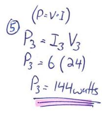
How much power is used by the unknown resistor?
