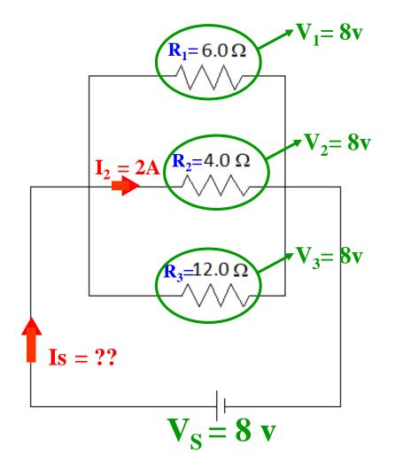
$\frac{\text{METHOD 1}}{\text{Step:1}}$   $V_{2} = I_{2}R_{2}$   $V_{2} = 2 (4)$   $V_{2} = 8 V$   $\frac{\text{Step:2}}{2}$
