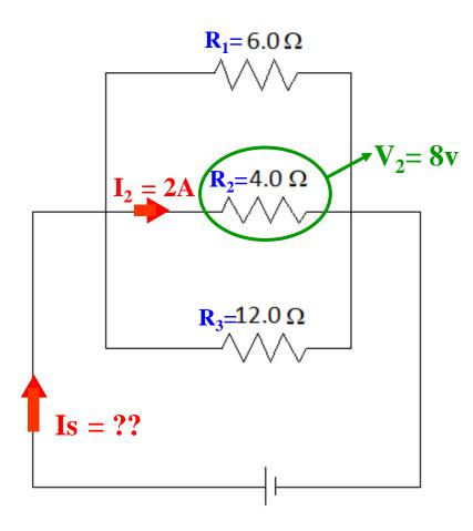
Step:1  $\mathbf{V}_2 = \mathbf{I}_2 \mathbf{R}_2$  $V_2 = 2(4)$  $V_2 = 8 V$ Step:2  $\mathbf{V}_{\mathrm{S}} = \mathbf{V}_{1} = \mathbf{V}_{2} = \mathbf{V}_{3}$ Parallel  $V_s = 8 V$
